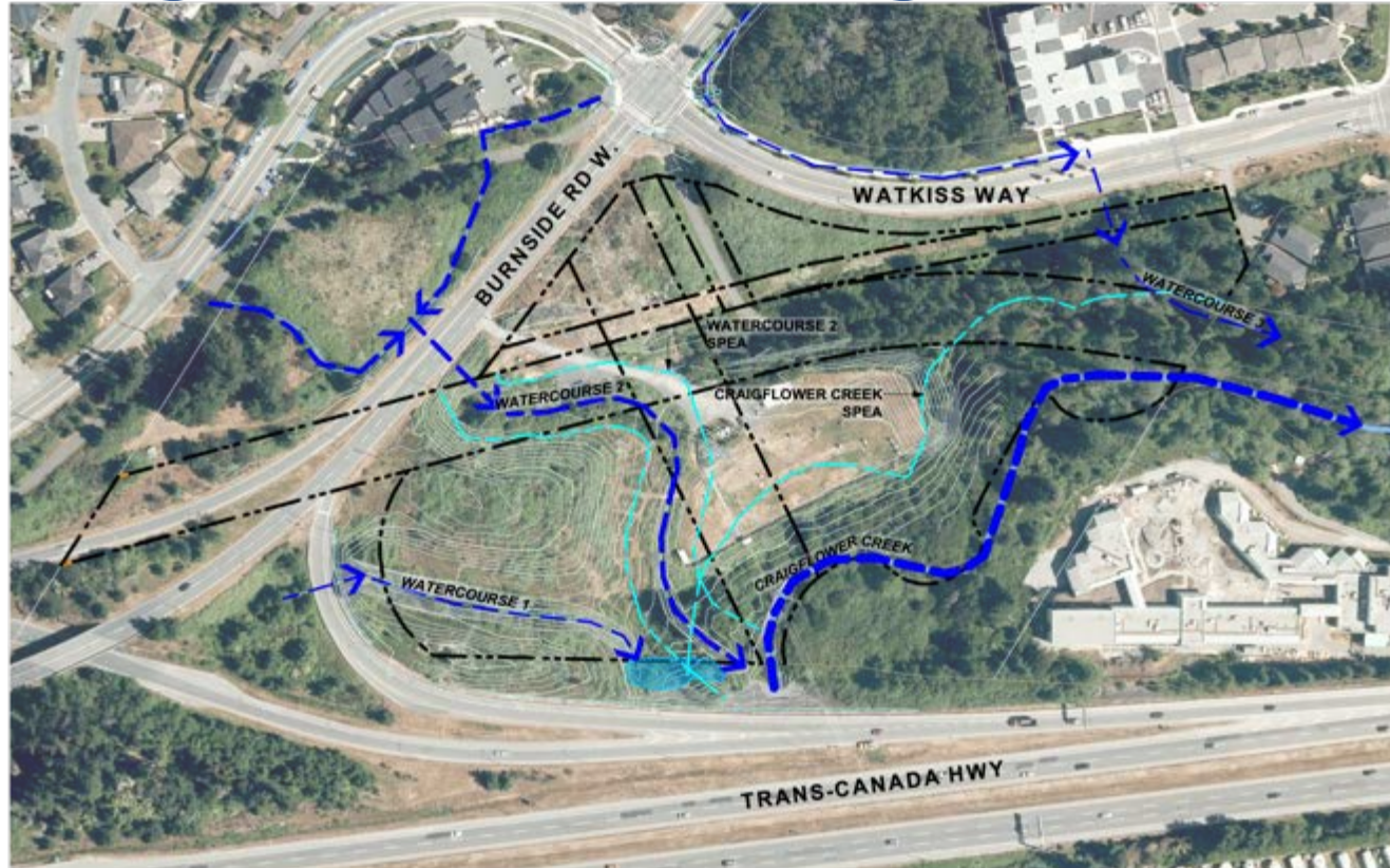
BC TRANSIT HandyDART EXISTING SITE DRAINAGE 1:1500
