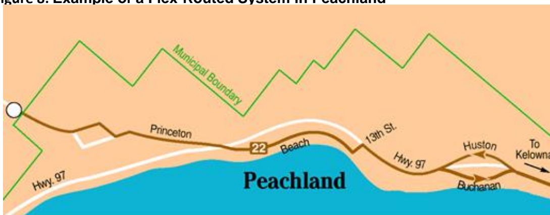
Figure 8: Example of a Flex-Routed System in Peachland
