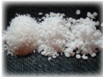
Filter media is available in fine (32-8), medium (8-4), and coarse (4-2) grades
